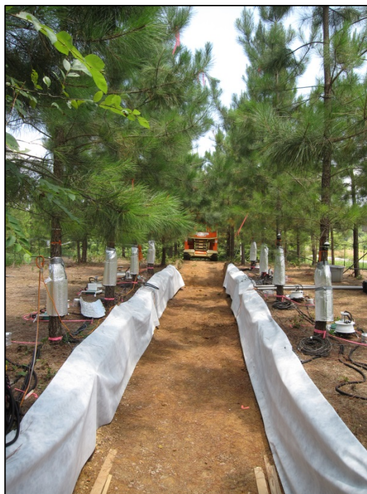
Figure 1. The PiTS-1 experimental plots were established across two rows in a stand of loblolly pine trees, with four adjacent sample trees selected from each row. A trench was excavated in-between the two rows and instrumentation installed as shown.
