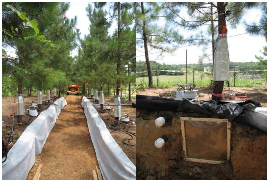
Figure 2. Experimental plot photographs: (a) trench excavated in-between the two rows of four trees, (b) completed installation of minirhizotron tubes, rhizotron windows, installed sap flow sensors, and static gas exchange chambers.
