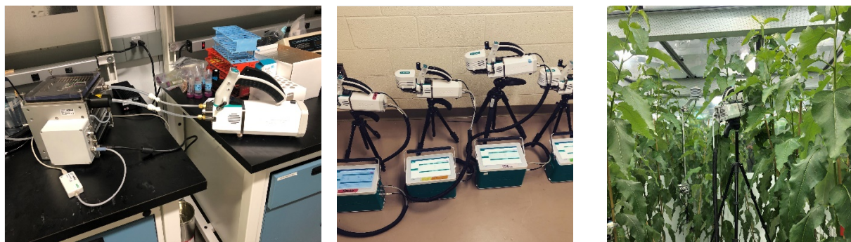
Figure 1. Leaf and root gas exchange measurements were conducted using the Li-6800 portable photosynthesis system. Left: the Li-6800 attached to the Walz respiration chamber, which was used to measure root tissue respiration and its response to temperature. Middle: fleet of Li-6800s ready to collected coupled leaf gas exchange and chlorophyll fluorescence measurements. Right: two Li-6800's collecting data in a growth chamber at Oak Ridge National Lab in Building 1506.
