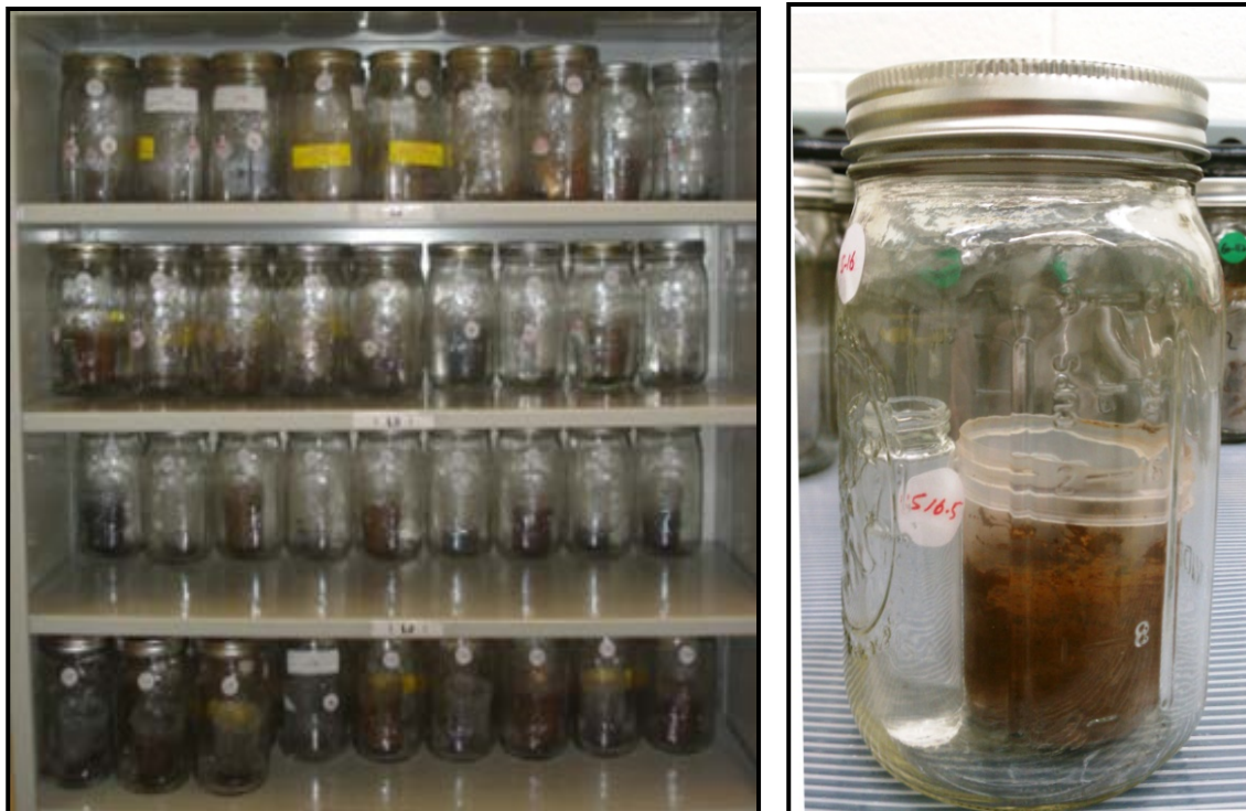
Figure 1. Left: Laboratory set up of incubation jars. Right: Close up of microcosm containing soil in specimen cup and CO 2 trap in glass vial.
