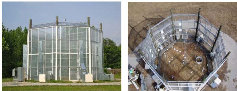
Figure 3. SPRUCE ecosystem warming enclosure concept (upper figure) and the final fully instrumented prototype (photographs). The warming enclosure has instrumentation for measuring turbulence, air temperature and relative humidity at multiple heights, and soil temperatures to depths as much as – 2m. Sampling tubes for [CO 2 ] measurements are also installed. Open path CO 2 and CH 4 sensors with sonic anemometers are currently being added (June/July 2011) to the central tower for “eddy-covariance-style” observations of the enclosure footprint.
