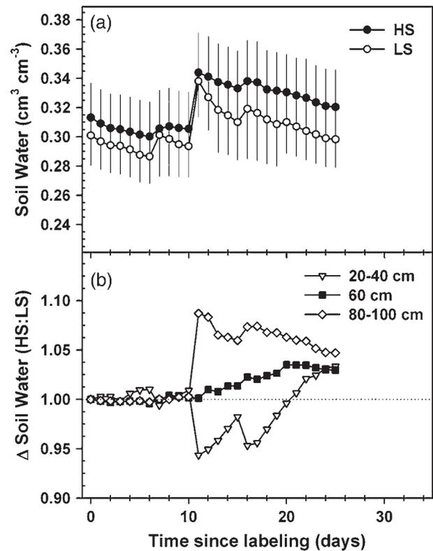
Figure 4. (a) Mean soil water content for the upper 1 m of soil (5–105 cm) after initiation of light shade (LS) or heavy shade (HS) treatments of loblolly pine trees ( $n = 4 \pm \text{SE}$ ). (b) Relative change in soil water content at different depth increments through time. Data from each sensor were normalized to 1 at Day 0. Values above 1 indicate greater water removal from the LS soil as compared with the HS soil.
