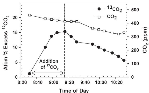
Figure 1. Change in atmospheric  $^{13}\text{CO}_2$  and  $\text{CO}_2$  within a translucent plastic chamber enclosing eight loblolly pines during a 2-h  $^{13}\text{CO}_2$ -labeling event in early September 2010.
